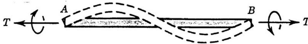
**Fig. 9.9** Twist-bend buckling of a shaft in torsion.
